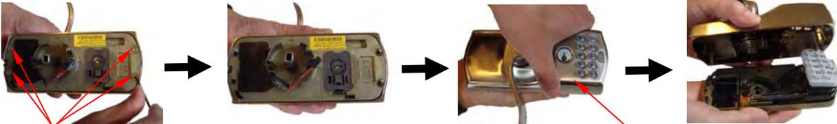
Remove the 4 screws using T15 Torx screwdriver
