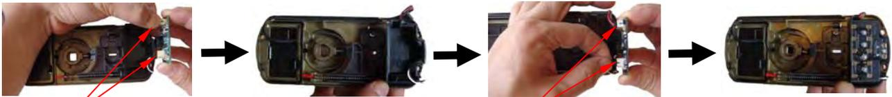
Disconnect the two connectors from old board
