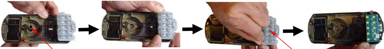
Remove the transmission shaft
